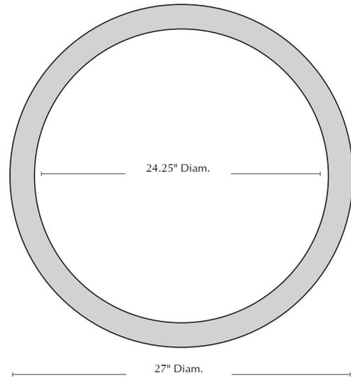
**Materials:** water, sand, stone aggregate and cement
