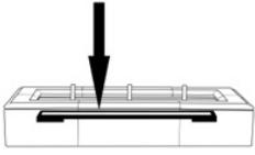
**Step 10** – Place the plate base (FT-427B) over the Pipe Assembly with the pump outside of the base.
