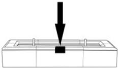
**Step 11** – Place the pump cover (FT-427C) over the pump and against the side wall of the basin.
